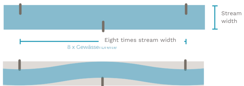
Figure 10: Added wood structures in top view, spacing between two elements on the same stream bank equals eight times the width; top: initial state, below: stimulated development.
